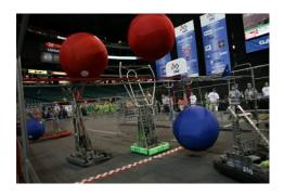
In the 2008 game, "FIRST Overdrive," students' robots are designed to race around a track knocking down 40" inflated Trackballs and moving them around the track, passing them either over or under a 6'6" overpass. Extra points are scored by robots positioning the Trackballs back on the overpass before the end of the 2 minute and 15 second match.
