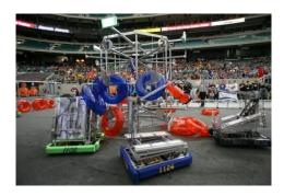
In the 2007 game, "Rack 'N' Roll," students' robots are designed to hang inflated colored tubes on pegs configured in rows and columns on a 10-foot high center "rack" structure. Extra points are scored by robots being in their home zone and lifted more than 4" off the floor by another robot before the end of the 2 minute and 15 second match.
